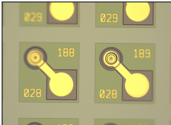
850 nm- 10G VCSEL (example device)
